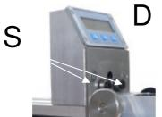
Send **only** the measuring case "**D**" to the manufacturer. For this reason unfasten the 2 countersunk screws "**S**" with the provided countersunk screwdriver and send the digital device "**D**" only to the engraved address.
